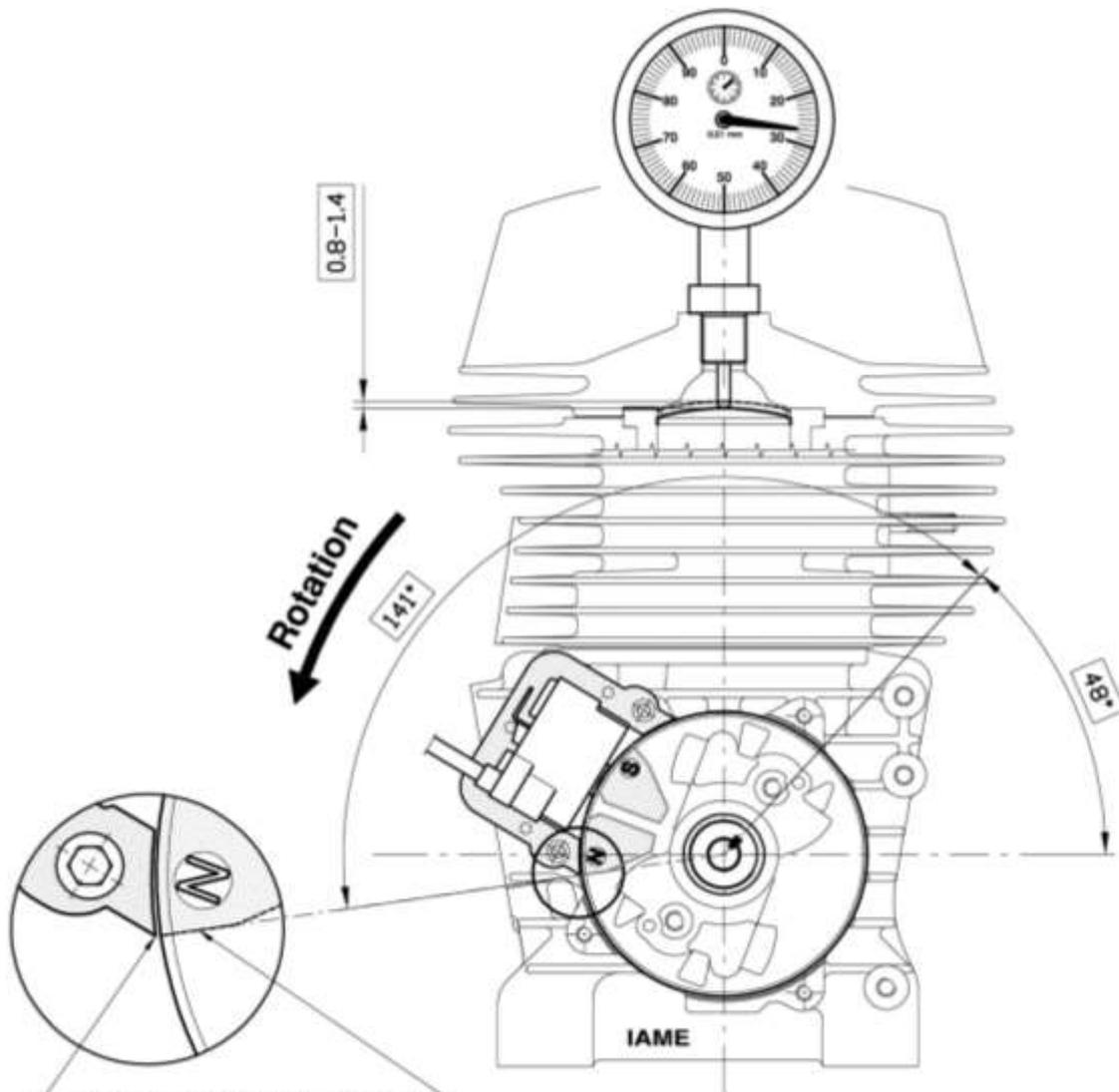
\* ALIGN THE ROTOR MAGNETO END ON THE IGNITION COIL END AS SHOWN.
